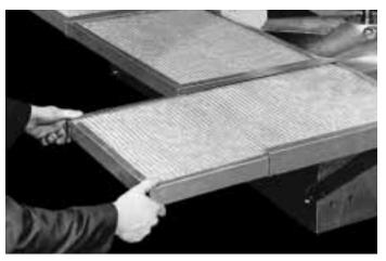
Sliding filter out of filter rack.
